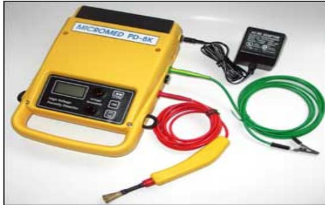
Develop a policy and procedure to visually inspect insulation each time with a lighted magnifying lamp. Look for cracks, holes, or flaking in insulation. Then follow with insulation testing equipment. All such testing should be documented on a log form. These records should be retained with the sterilization records.
