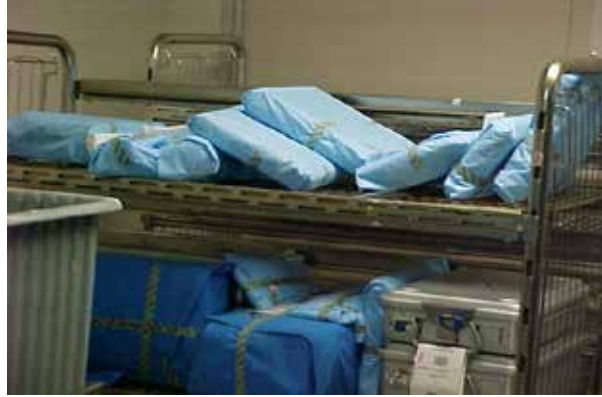
INCORRECT loading of sterilizer; trays stacked, items too close.
