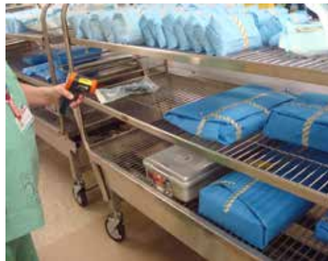
Infrared thermometer gun to determine the temperature of packs before handling
