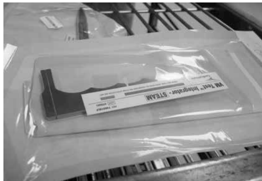
Photo Above – Incorrect Packaging - Paper-Plastic Pouch Doubled, Inside Pouch Folded Over
