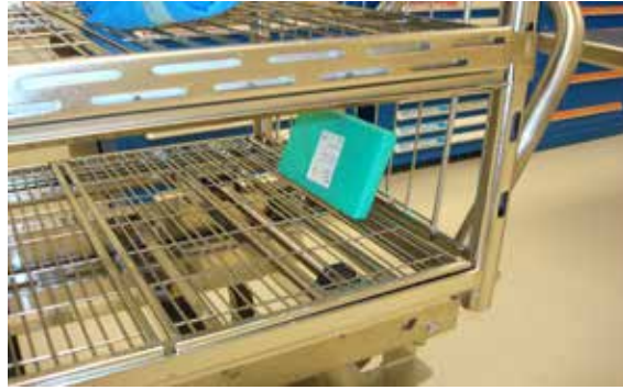
Photo Above – BI PCD not placed flat, or over the drain line as required
