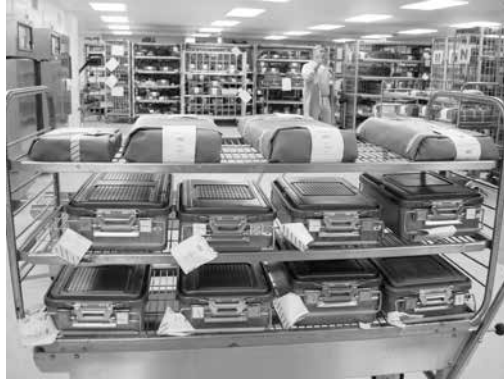
Photo Above - Correct Loading of Steam Sterilizer
