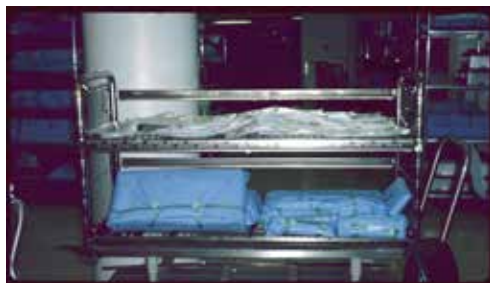
Photos Above – Incorrect Loading of Steam Sterilizer
