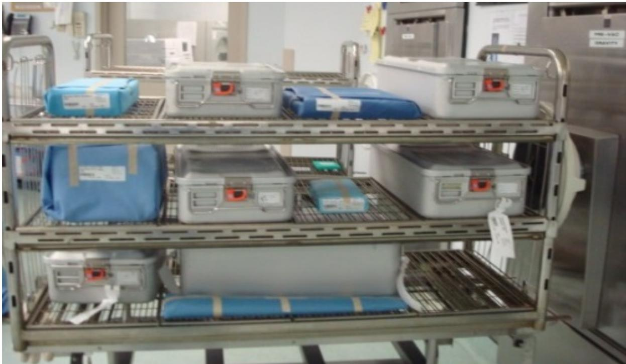
**Photo Above - Maximum Load Test Loading of the Sterilizer. Note the 2 containers on each shelf that contain the BIs.**
