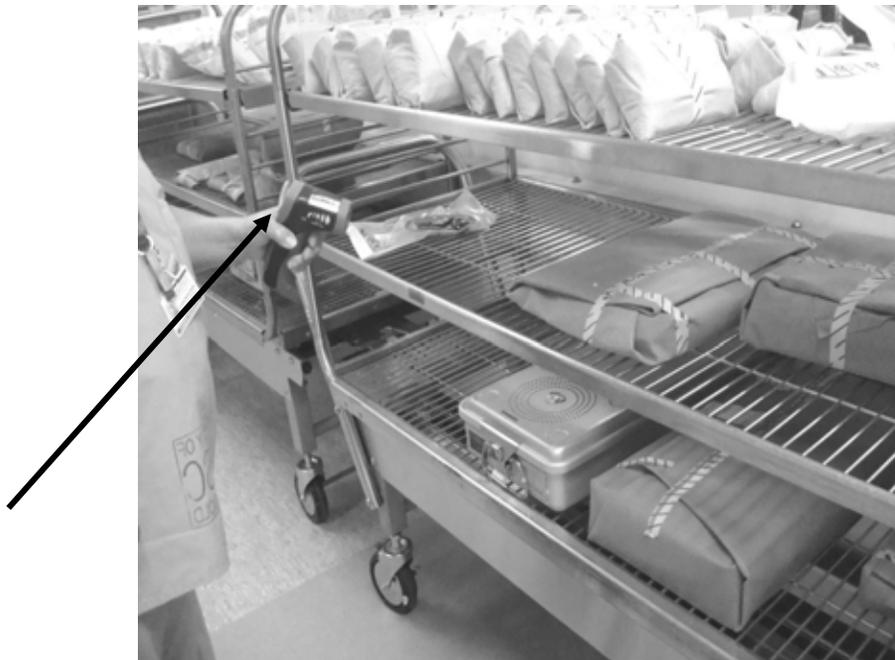
**PHOTO ABOVE - Arrow pointing to an infrared thermometer gun to measure the temperature of each pack**
